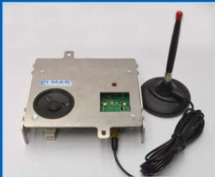
The information (digital/analogue signal) is processed by one or more modules provided with microprocessor, by means of electronic devices (optocouplers, infrared passive sensors, thermo-resistors, capacitive microphones, galvanic transformers, etc.). The radio module (GSM/GPRS/PCS) transforms the communication protocols in radio waves of 900/1800/1900 Mhz, and, at the other end, at the reception point, decoding and converting the signals in a database compatible with the PC system take place.
